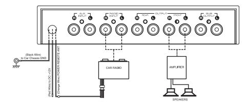
Connect the Radio/CD source unit to the Radio Input jacks. Make sure the Source input selector switch on the AEQ-4XOA front panel is in the correct position. Likewise, if only one set of RCA cables are run to your amplifier(s), make sure the Fader control is turned to the direction that gives you output to the jacks being used (clockwise for rear, counter-clockwise for front).
