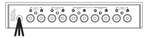
1) Power Wires: Connect the three pigtail wires from the rear of the EQ as follows
