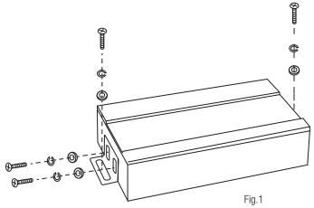
There are two basic mounting options for your PowerBass Line Output Converter. One is to mount the unit using the supplied brackets as shown in Fig 1. Once attached, you may use the brackets as a template and mark the two screw locations with a felt tip pen. Use caution to make sure there are no objects behind the installation surface that may become damaged during drilling.
